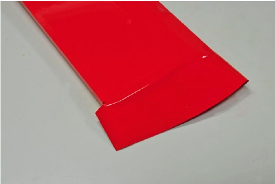
Using the trim iron, tack the covering at one end to the rib just inside the black mark. Later, you can remove the black mark with alcohol. Grabbing the loose end, pull it across the top of the rib for an even-width seam, and iron in place. You are now ready to tack and iron down the opposite side.
