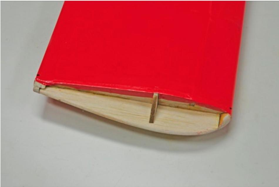
On the piece of covering to be applied, develop a contour to fit the rib for an even overlap seam, generally to the shape of the rib contour. The overlap should be approximately 1/4 inch.
